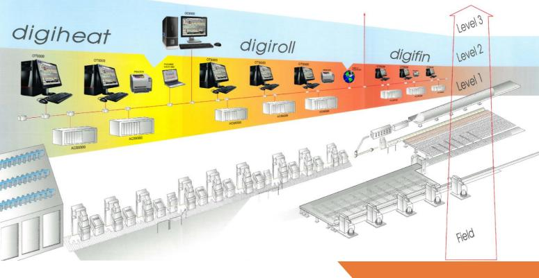
The DIGIROLL system permits the visualization of graphic diagram, pie-chart, bar graph of plant status in real-time.
